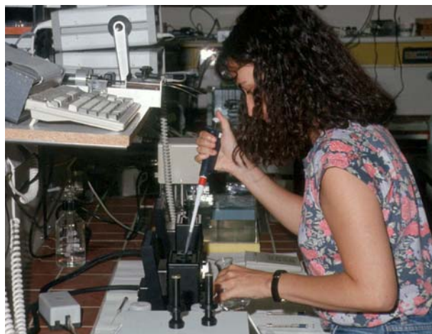
IOC01: Gabriela Méndez injects isolated rat liver mitochondria into the chamber of the Oroboros Oxygraph (O2P, Paar, Graz) at the International Summer Course, Innsbruck 1991.
